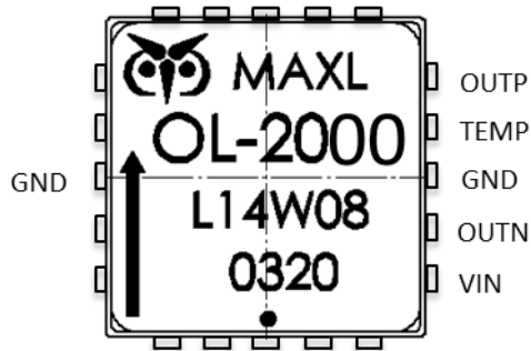
Figure 2 Pinout Description (Top View)
