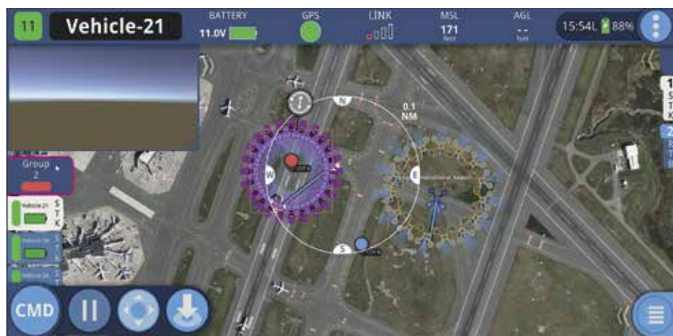
Autonodyne's software manages numerous UAVs using automated behaviour profiles
