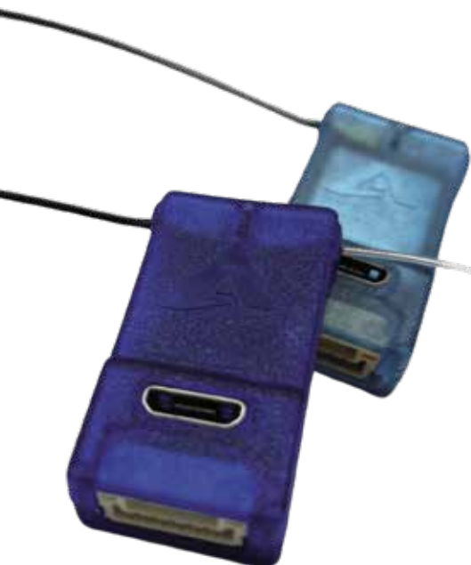
Aerobits' remote UAV identification systems
